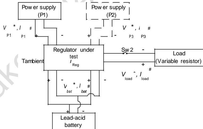
NOTE Power supplies 1 and 2 have on-board voltage and current measurement
