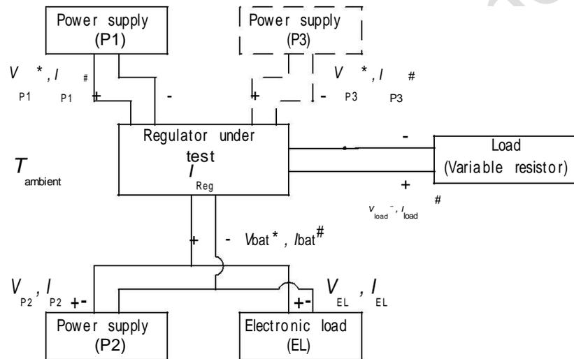
NOTE 1 Power supplies, 1, 2 and electronic load have on board voltage and current measurement.
