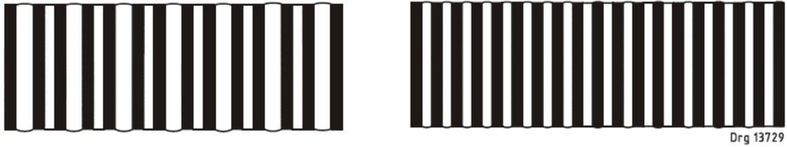
**Figure 1(b) Examples of an incorrect strobe pattern**
