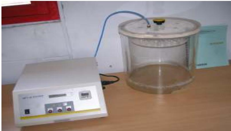
**Fig-8. Air proof leakage tester**
