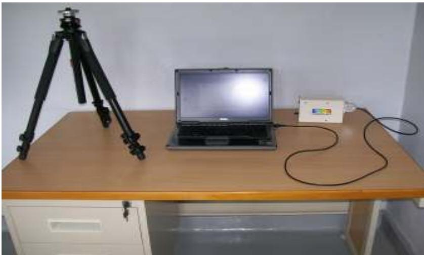
*Fig-10. StellarNet EPP2000C UV-VIS Spectrometer*
