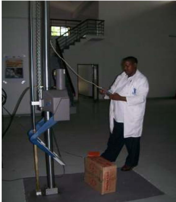
**Fig-4. Packaging Technologist working with drop tester
