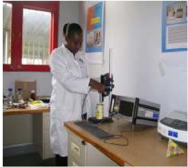
*Fig-7 b) Food packaging technologist working with Oxysensor at the food packaging laboratory*
