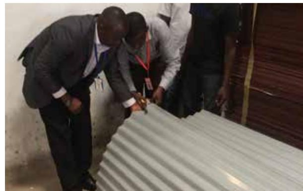
*TBS inspectors destroy substandard roofing sheets.*
