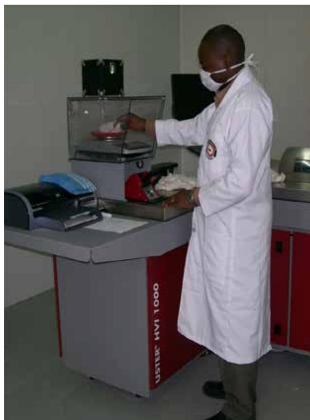
*High Volume Instrument (HVI) at TBS Cotton Testing Laboratory*
