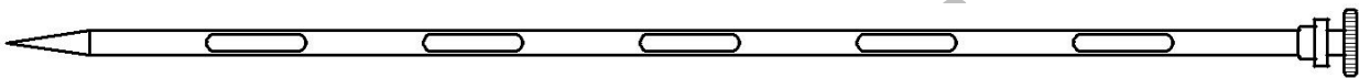
Figure B.2 — Open shaft with several apertures or closed shaft with compartments and several apertures
