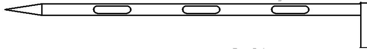
Figure B.9 — “Walking stick”-type, concentric sampling probe for sacks: open shaft with several compartments
