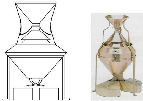
Figure B.14 — Cone-shaped divider (Boerner type)
