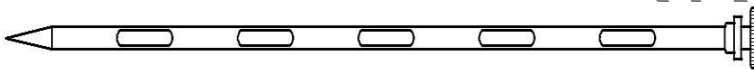
Figure B.2 — Open shaft with several apertures or closed shaft with compartments and several apertures
