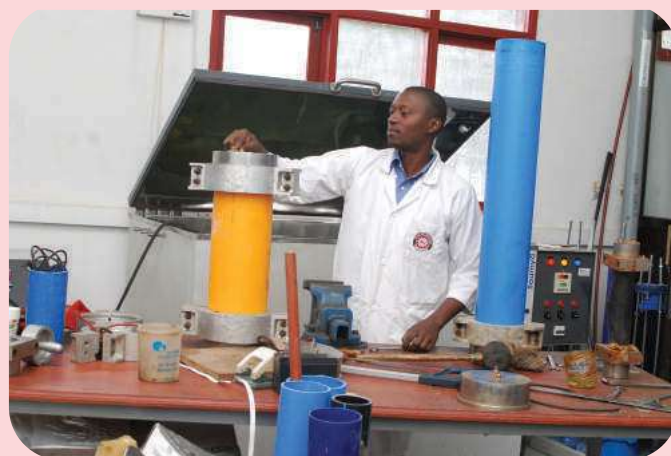
Testing of plastic pipes in the Building and Construction Laboratory
