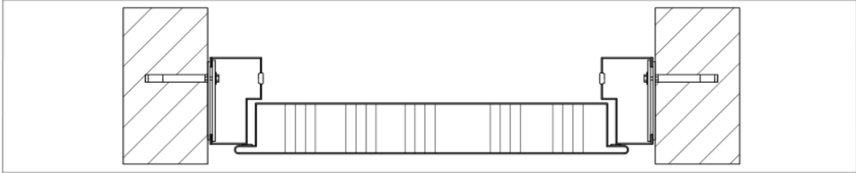
Figure B.3 Typical over-rebated doorset
