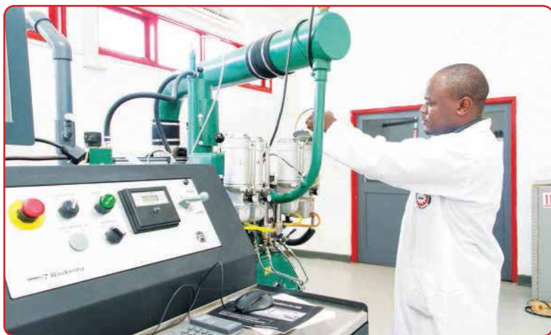
The CFR machine used to test Research Octane Number (RON) in petrol
